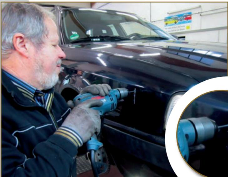
Increase the size of the middle hole to 25.7 mm. Using a step drill might help you. Enlarge the hole at the left and right side with a file so that the base and its 2 bolts will fit.
